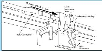
FIG. 6-2 Engage Chain/Belt Connector to Carriage.
